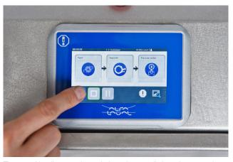
The user-friendly control panel. Just choose oil viscosity, press the start button and the system operates without supervision.
